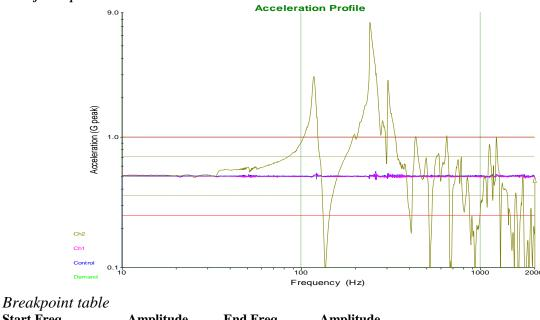
Start Freq. Amplitude End Freq. Amplitude 10 Hz 0.5 G 2000 Hz 0.5 G
